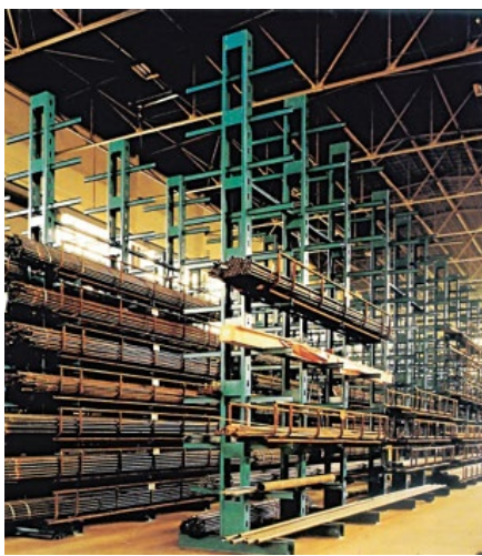
Fig. 4. Example of cantilever racking
