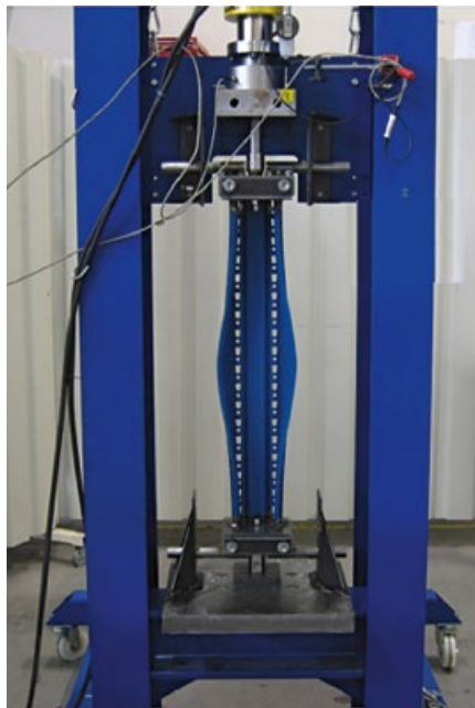
Fig. 15. Distortional buckling of an upright
