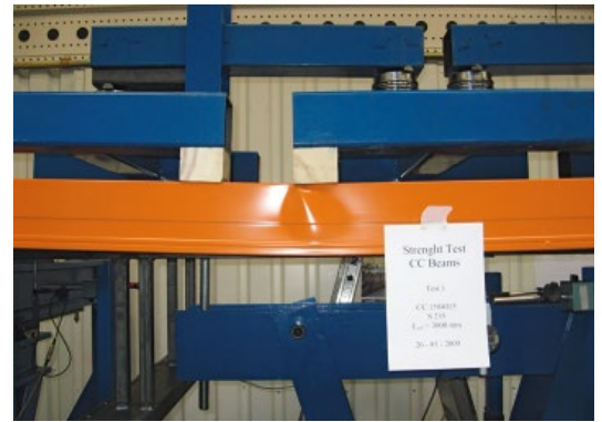
Fig. 25. Simulation of concentrated load transfer via the timber blocks of a pallet, causing additional crippling effects
