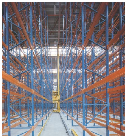
Fig. 6. Pallet rack operated by stacker crane
