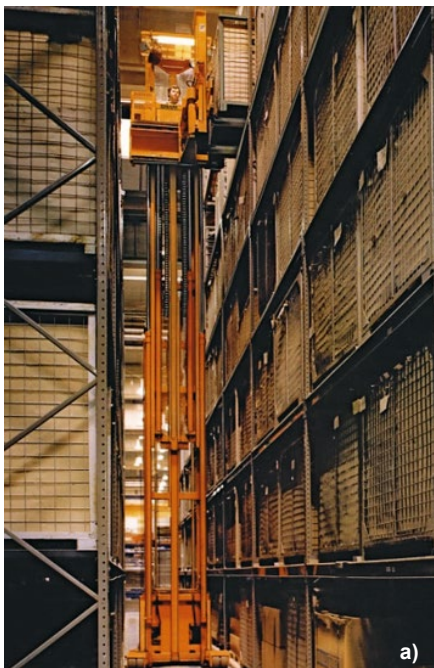
Fig. 5. Pallet rack operated by very narrow aisle truck: a) "man-up" operation, b) dynamic effects when travelling and lifting simultaneously
