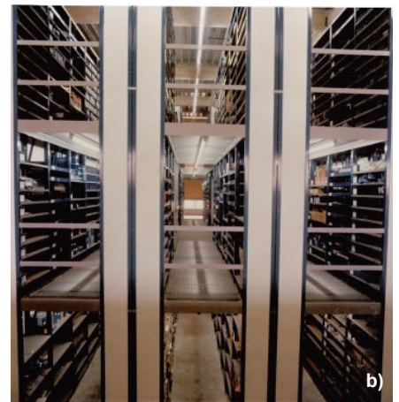
Fig. 7. a) Sketch of multi-tier shelving system; b) Example of 3-level multi-tier shelving
