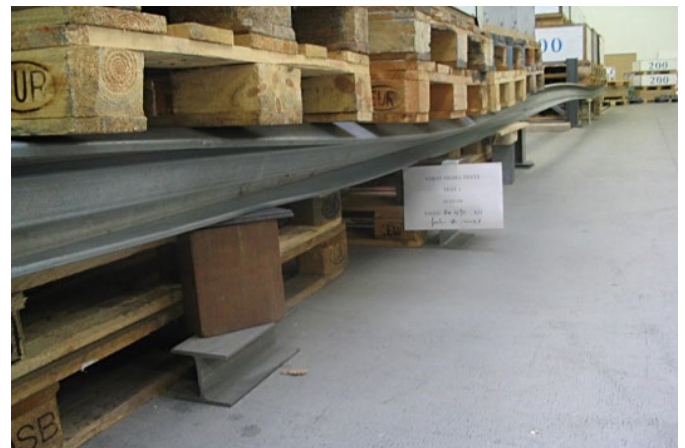
Fig. 26c. Design assisted by testing to determine ultimate load of \Sigma -beam, including all effects
