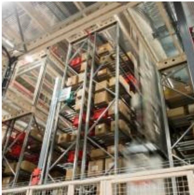
Figure 2 D Automated “small part shuttle racking”, is becoming more and more important because of the web shops and also requiring very tight floor deformations
